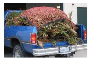
Incorrect and unsafe way of securing loads (above); items may fly out of or drop off of loads with the potential to strike other vehicles and cause litter on roads or injury to other drivers.
