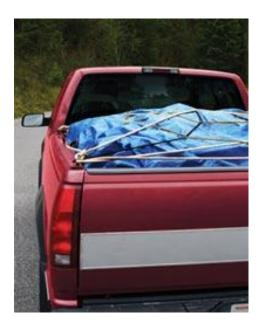
The safest way to secure your load; low in the vehicle, covered with a tarp; tied down and attached to the vehicle.
